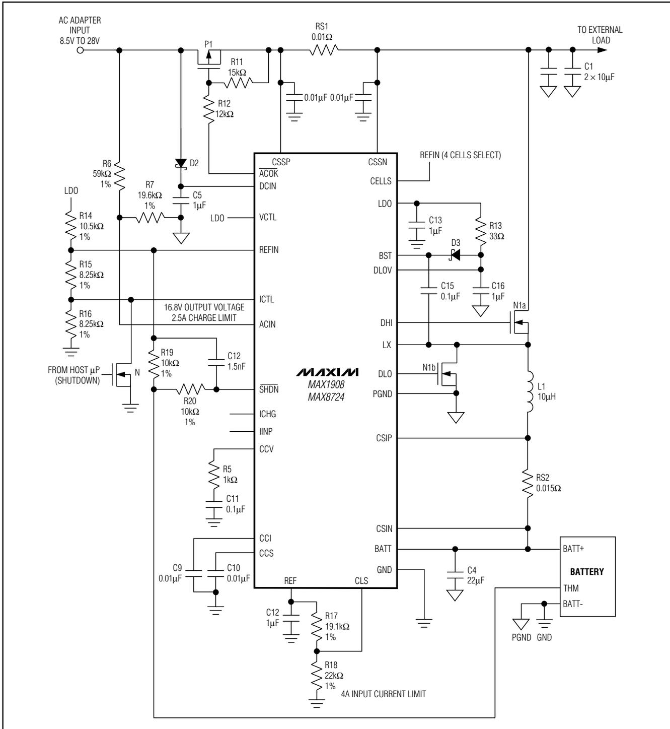
Figure 2. Typical Application Circuit with Fixed Charging Parameters
