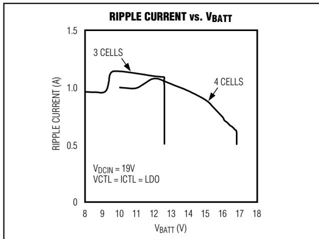
Figure 11. MAX1908 Ripple Current vs. Battery Voltage
